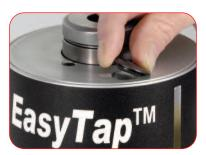
Has automatic lubrication system which dispenses pre-set amount of lubrication to the tap point with each tapping cycle. Built in sight gauge shows lubrication level.
